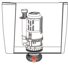
5.Insert the tank to bowl rubber gasket on to the flush valve's outlet bottom.
