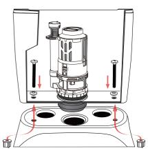
6. Insert the tank to bowl with one pair of plastic or stainless steel bolts through the holes. Insert washers on bolts and screw on the nuts.
