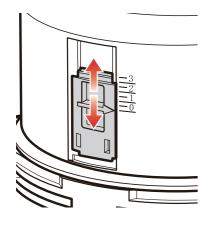
7.Adjust the full flush volume by sliding the red part up or down. when the buoy is higher, the discharge water volume is less, slide down the part can buoy little until you are flushing enough water.
