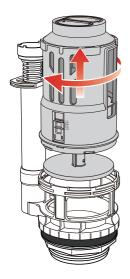
1. Hold the base of the flush valve and rotate the body counterclockwise Take it out from base.
