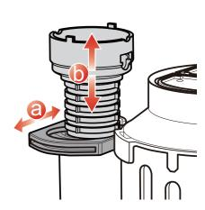
9. To adjust the height of the overflow pipe, slide the lock(a), then set the desired height of the overflow pipe(b). Put the lock back after.
