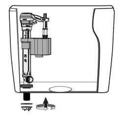
2. Position the fill valve with rubber gasket into the inlet hole of water tank and screw the lock nut with collar tightly. Caution!!! Do not over tighten the nut.
