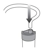
4. Attach one end of the refill tube to the overflow pipe, and the other to nipple located near top of valve.
