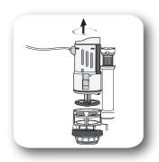
Hold the base of the flush valve and rotate the body counter-clockwise.
