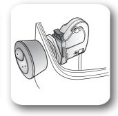
5. Install dual flush button in the flush handle hole. See "Button installation" for side hole or top hole installation.
