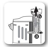
8. To adjust the height of the overflow pipe, slide the lock (a), then set the desired height of the overflow pipe(b). To fix the pipe with the lock part.
