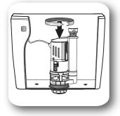
4. Take the body of flush valve and set it into the base and lock in place by rotating it clockwise.
