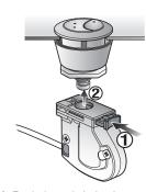
3. Push in switch box's green button(1) to connect with button body.
