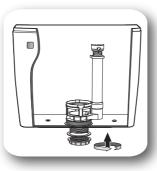
Position the flush valve's base into the water tank. Screw on the nut collar and hex nut properly.
