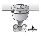
2. Insert the button into the oval hole of tank,then screw up subcover, flanged nut in sequence.
