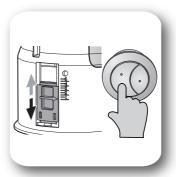
10. Press Full Flush button. Ensure bowl empties sufficiently, and siphon action is activated. If siphon action is not activated, adjust Full flush setting (red) down one notch to 4.5. Press Full Flush button again. Repeat this process until bowl empties and siphon action is activated.
