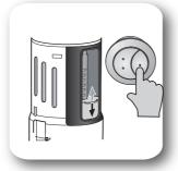
9. Press half Flush button. Ensure that bowl empties sufficiently, and siphon action is activated. If siphon action is not activated, adjust half flush setting (blue) down one notch to 8.5. Press half Flush button again. Repeat this process until the siphon action is activated.
