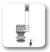
Remove the hex nut and nut collar form flush valve base. Don't remove the seal.
