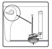
5.On the basis of form a complete set of lever installation instructions, install the tank lever in the toilet water tank corresponding assem bly position.
