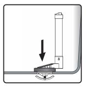
2.Position flush valve into the mounting hole.
