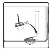
4.Connect the flapper to flush valve.
