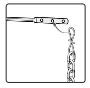
6.Connect the flapper chain. Allow slight slack when flapper is in closed position.
