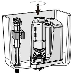
19. Position the valve body into the base and lock it in place by rotating it clockwise.
