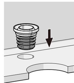
14. Install the tower-shape gasket into the tank hole.
