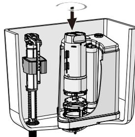
19. Position the valve body into the base and lock it in place by rotating it clockwise.
