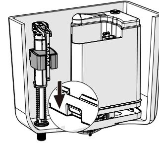
18. Position the tank body onto the base.
