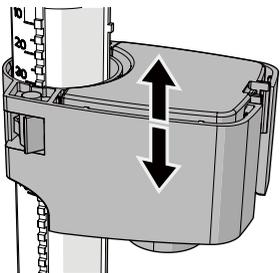
7. Pull the buoy up and down until adjusting to the suitable height.
