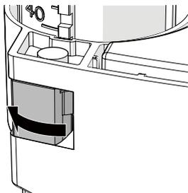
8. Turn the lock buckle to the locked position.
