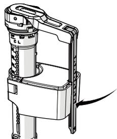
9. Inward to lock the float lever to lock.
