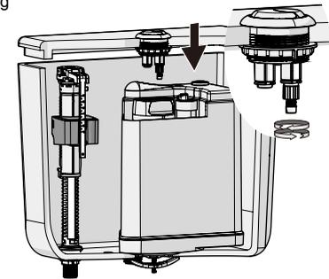
24. Position the ceramic tank cover onto the tank. Remarks: Loosen the nut, adjust the rod to the suitable length, screw up the bottom nut tightly.
