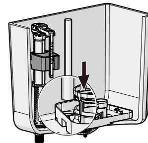
17. Insert the pipe into the tank hole. Remarks: The pipe should be inserted to the bottom of the tower-shape gasket.
