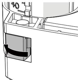
8. Turn the lock buckle to the locked position.
