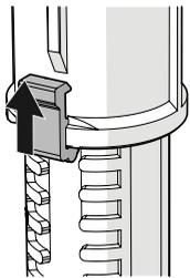
4. Push up into the buckle to the locked position.
