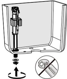
11. Install the fill valve into tank, rotate the gasket and nut.
