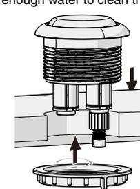
23. Position the button body into the ceramic hole. Make sure the button rod aim at the full-flush part, screw up the bottom nut tightly.
