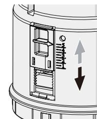
20. Adjust the full flush volume by sliding the buoy up or down. When the buoy is higher, the water is less and the flush time is shorter. Slide the buoy down little by little until you are flushing enough water to clean the bowl.
