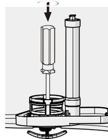
16. Position the base into the ceramic hole. use screwdriver to screw up the nut tightly.
