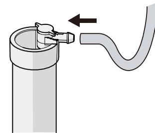
21. Attach the refill tube to the overflow pipe for refill.
