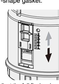
20. Adjust the full flush volume by sliding the buoy up or down. When the buoy is higher, the water is less and the flush time is shorter. Slide the buoy down little by little until you are flushing enough water to clean the bowl.
