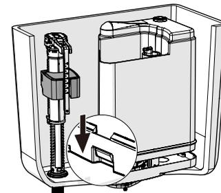
18. Position the tank body onto the base.
