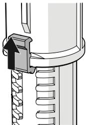
4. Push up into the buckle to the locked position.
