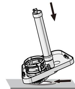
15. Position flush valve base into the mounting hole.
