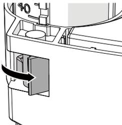
6. Rotate the buoy of lock buckle.
