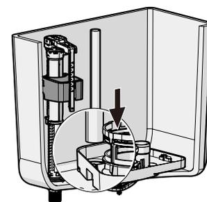
17. Insert the pipe into the tank hole. Remarks: The pipe should be inserted to the bottom of the tower-shape gasket.
