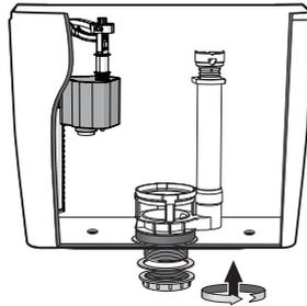
3. Insert the flush valve's base with rubber into the water tank, then screw on the plastic nut collar and hex nut properly.
