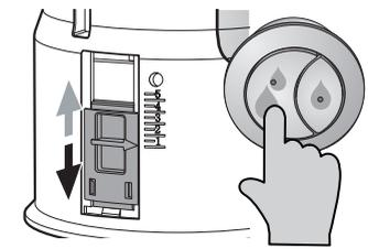
8. Press Full Flush button (2 water drops). Ensure bowl empties sufficiently, and siphon action is activated. If siphon action is not activated, adjust Full flush setting (red) down one notch to 4.5. Press Full Flush button again. Repeat this process until bowl empties and siphon action is activated.
