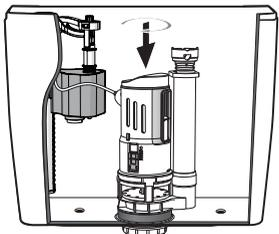
4. Take the body of flush valve and set it into the base and lock in place by rotating it clockwise.
