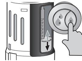
7. Press 1/2 Flush button (1 water drop). Ensure that bowl empties sufficiently, and siphon action is activated. If siphon action is not activated, adjust 1/2 flush setting (blue) down one notch to 8.5. Press 1/2 Flush button again. Repeat this process until the siphon action is activated.
