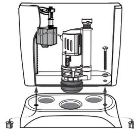
6. Take the water tank and install it on the two piece toilet of mounting holes, then fasten the bolts.
