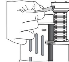
10. Insert the filling water hose of 10mm length into the overflow pipe inside.
