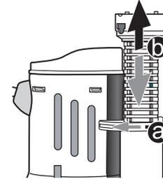
9. To adjust the height of the overflow pipe, slide the lock (a), then set the desired height of the overflow pipe (b). Put the lock back after.
