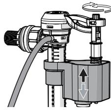
3. Adjust the screw to adjust the water level to the proper line inside the tank.
