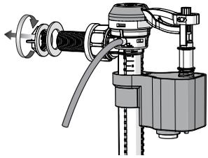
1. Disassemble the lock nut, Plastic washer, Coupling nut for valve installation.
