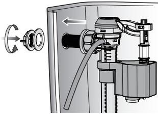
2. Position the fill valve with rubber gasket into the inlet hole of water tank and screw the lock nut with collar tightly. Caution!!! Do not over tighten the nut.
